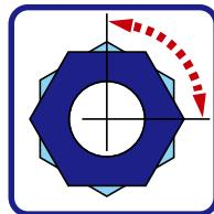
The tightening torque is displayed as an angle.
